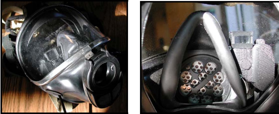
Figure 3: Exterior and interior of SCBA facemask. The head-mounted display can be seen in the lower left (exterior) and lower right (interior). The interior picture demonstrates how the LCD screen is translucent when turned off.
